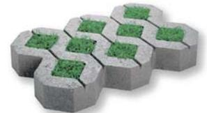
Turfstone is a large paving unit with openings that can be planted with grass to provide a "green" pavement or can be filled with stone to help manage stormwater runoff and allow for the infiltration of rainwater. For information on the installation of Turfstone pavements, contact **Ideal**.
